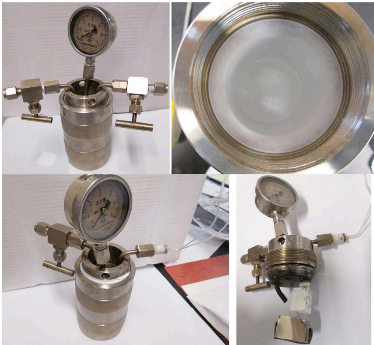
Fig. S4. High-pressure cell used to measure saturated water pressure as a function of temperature. The Tech-zoom stainless steel reactor has an inner 200ml Teflon chamber (top shown as used to measure saturated steel water pressure), and (bottom) is shown as in-house modified for electrolysis by replacement of the right-hand flow valve with throughput electrical contacts using an OMEGA MFT-116-3 Feedthrough for up to three 1/16” diameter probes with a ¼” NPTM fitting.
