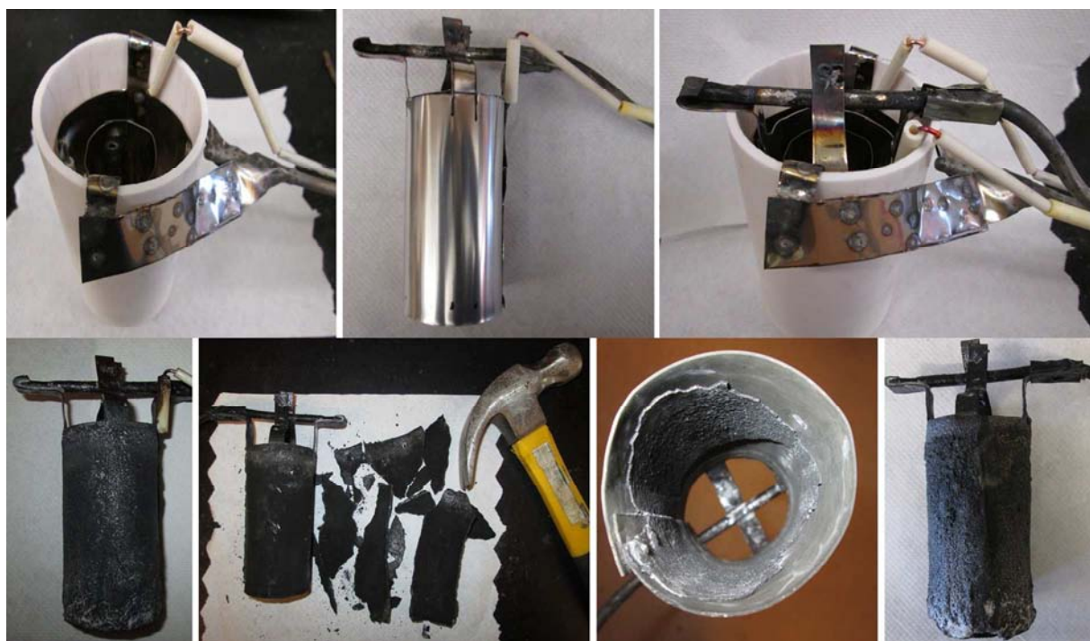
Figure S7. Scaled-up electrolysis chamber splitting CO 2 operated at 100 amp. Driven with a Xantrex XTR 0-100 A DC power supply, 1.5V, and approaching 100% coulombic efficiency of the 4 electron reduction to carbon.
