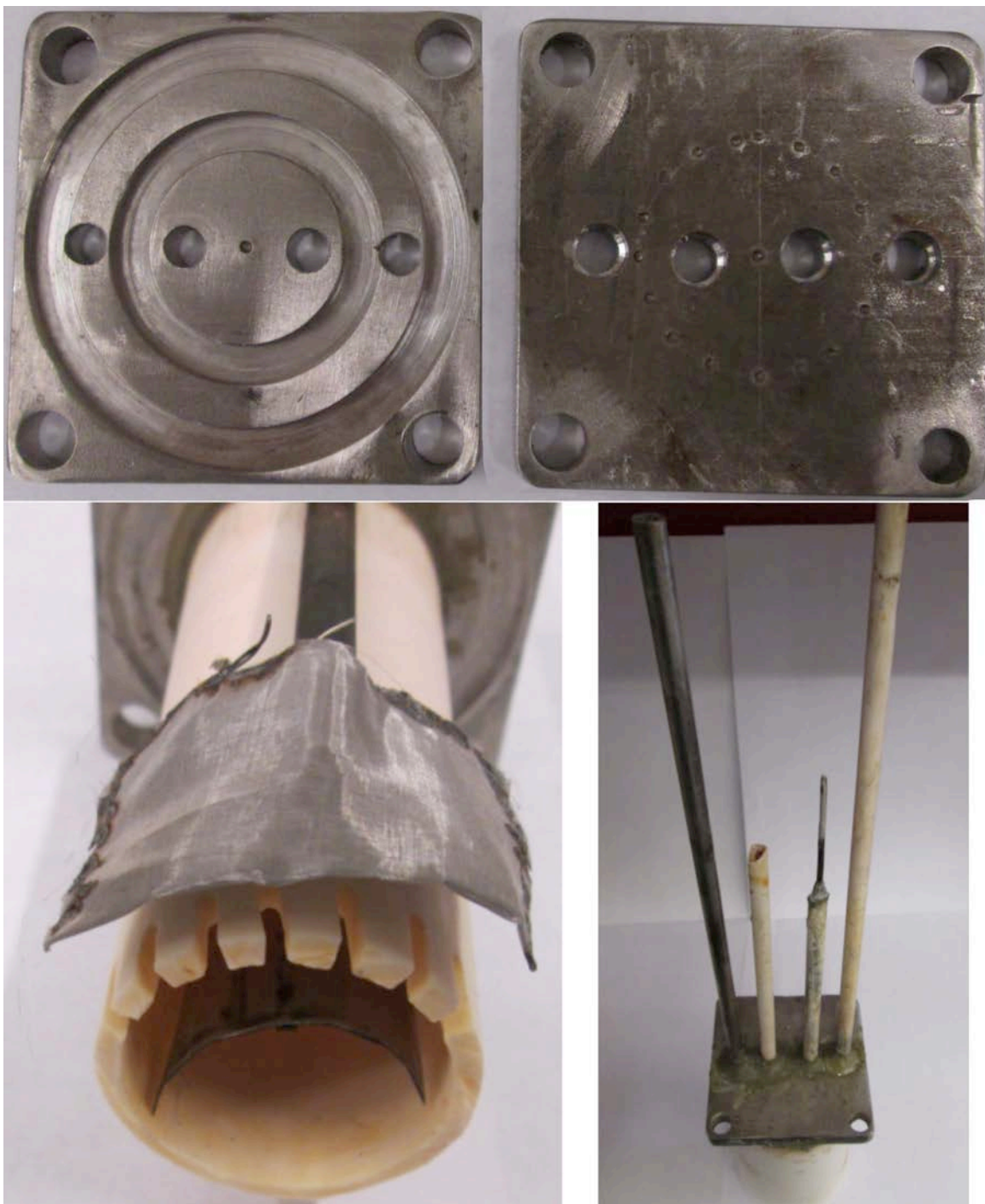
Fig. S2. The double chamber electrolysis cell configuration as described in the text and used to confirm that ammonia was produced at the cathode and oxygen at the electrode. Top left and right photos: underside and top of cell cover. Bottom photos, left: alumina tube with cathode outside and anode inside, prior to addition of electrolyte and outer crucible. Right: Double chamber cell prior to closure with bolts showing from right to left inconel tube for gas inlet & cathode electrical connection, outer chamber gas outlet, inner chamber electrical connection to anode, and inner chamber gas outlet.
