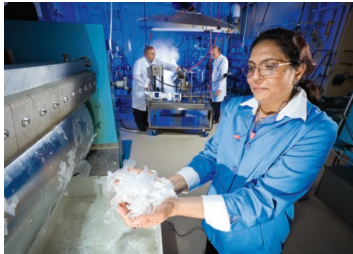
The FANTESK that food technologist Mukti Singh (foreground) examines as it comes off a drum dryer was prepared by plant physiologist Frederick Felker (background, left) and chemist George Fanta (background, right) using a steam jet cooker. Singh uses FANTESK to cut the fat and calories in cake and frosting.
